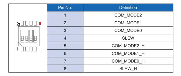
The COM1 and COM2 Ports Mode have to be changed by SW4 & SW5 respectively. Please refer to below figure the truth table of mode.
